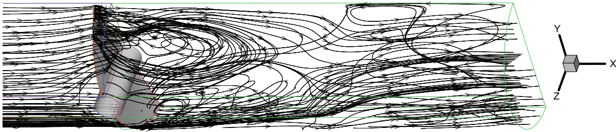
Fig. 8. Streamlines at the valve angle of 15^\circ .
