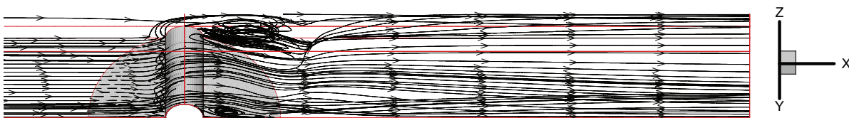
Fig. 11. Streamlines at the valve angle of 90^\circ .
